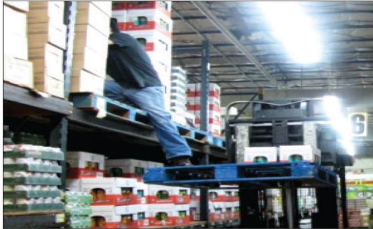
Figure 1: Example of a worker unsafely pulling inventory on a raised pallet.
